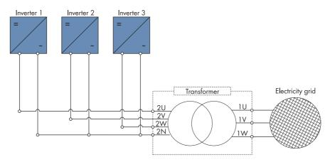
☐ The unbalanced load capacity of the transformer must be taken into account for operating the Sunny Boy and Sunny Mini Central single-phase inverters.
