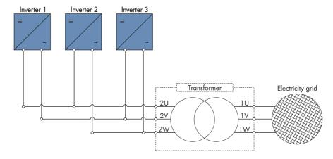
On a three-phase electricity grid, each of the following single-phase inverters can be operated between two line conductors if the neutral conductor is connected:
