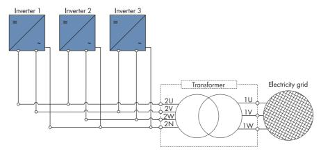
On a three-phase electricity grid, each of the following inverters can be operated between one line conductor and the neutral conductor:
