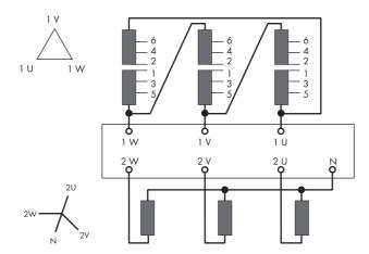
□ For inverters with transformers (Sunny Mini Central A, Sunny Mini Central HV, Sunny Boy US), SMA Solar Technology AG recommends transformers with a delta connection on the medium-voltage side and a star connection on the low-voltage side. A neutral point that leads outward is not required, e.g. Dy(n)1, Dy(n)5, Dy(n)11 (see figure below).
